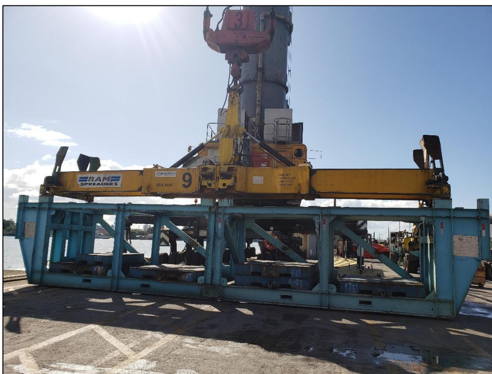
Figura 3. Teste de carga – Single Lift.
